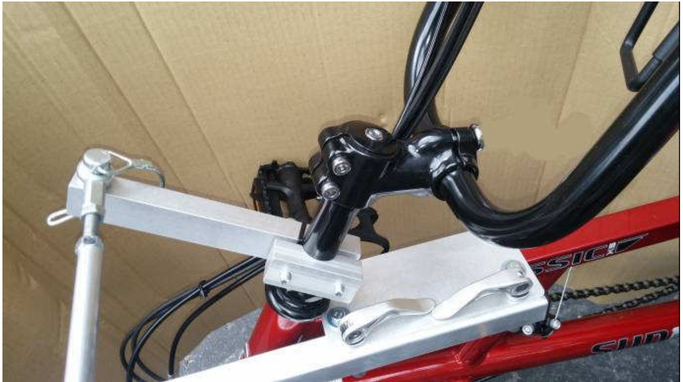
Removable steering tie rod, removable front beam.
